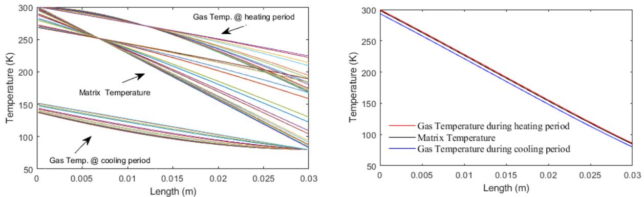
**Figure.2** Left: matrix and gas temperature variations during heating and cooling period, right: the final temperature profiles as they converge to solution with increasing  $N_x$  and  $N_t$ .
