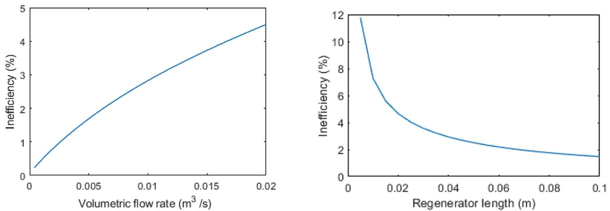
**Figure.3** Left: effect of increasing volumetric flow rate on  $I_e$ , right: the relation between the regenerator length and  $I_e$ .
