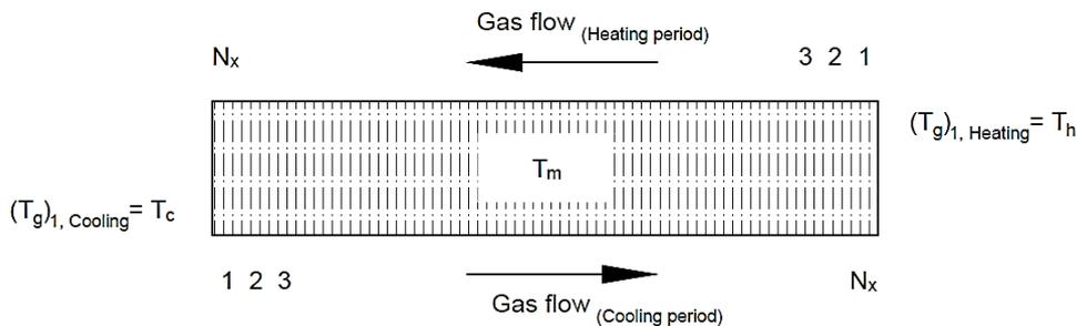
**Figure.1** Numerical schematic for the regenerator during heating and cooling periods, where  $N_x$  and  $N_t$  are the total number of spatial and time elements,  $T_h$  and  $T_c$  are the hot and cold temperature levels.
