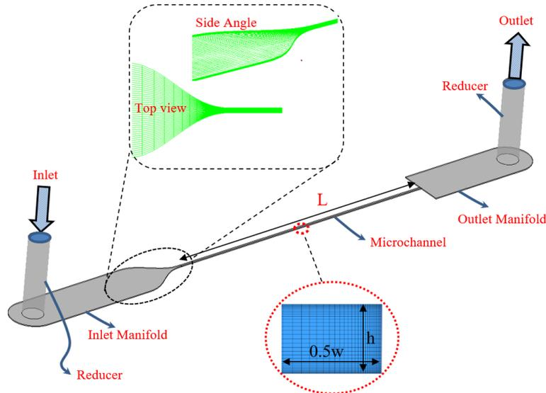
**Figure 2:** Geometric model used for numerical analysis of MC with bellmouth (BM) inlet.
