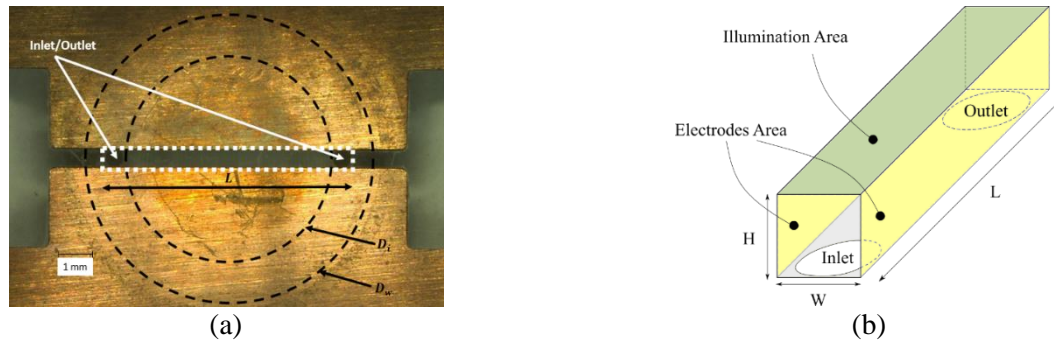
Figure 2: a) Optical microscope image indicating microchannel, illumination and window diameters; b) Microchannel schematics with main geometry and geometrical parameters.
